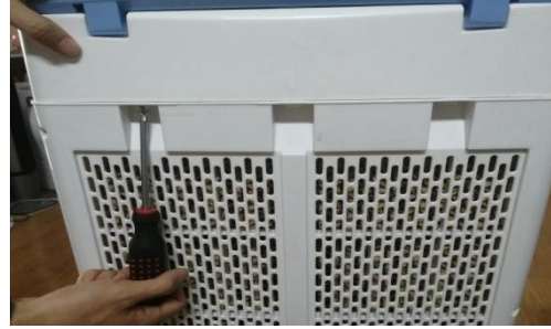
b. Remove the screw of back dust filter.
