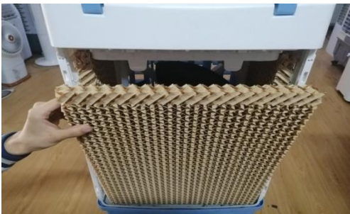
c. Gently take down the removed cooling pad to avoid damaging the cooling pad.
